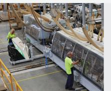
At Jayco, we are committed to investing in newer, more advanced technology. This allows us greater flexibility in producing exciting new layouts. For example, our million-dollar investment in the custom Italian-built Double Edge banding machine allows us to maximise operational efficiency by edging two sides at once.
