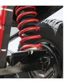
Purpose designed to complement the Jayco Endurance Chassis, JTECH Suspension replaces beam axles with individual stub axles, allowing each wheel to react independently to the road surface, while lessening the chassis' unsprung weight. JTECH Suspension makes towing easier and safer than ever before.
