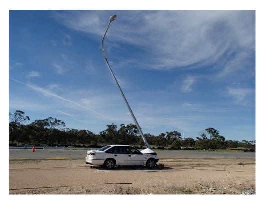
EASLP test photo. A car travelling at 60kph has been arrested by the Energy Absorbing Light Pole and is supporting the EASLP against the vehicle
