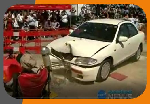
Televised crash testing of Energy Absorbing Bollards
