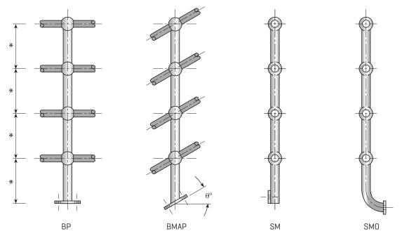
\*Specify number of balls, pitching & height required of stanchion (150mm minimum centres) Multi ball stanchions are available in any of the range of Balltube stanchion configurations
