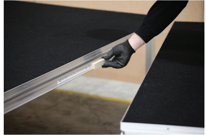
Insert Wood Block midway along the 1.5m Podium Extrusion - slide both Podiums together
