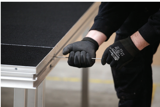
Using Klemm-fix Tool insert the Klemm-fix Connector in either side of the 2 Podiums flush with Extrusion
