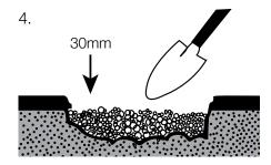
Leave in the sun for few minutes to improve ease of spreading. Evenly spread the material over the area in layers not exceeding 30mm.
