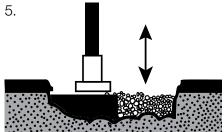
Compact using a roller, plate compactor or hand tamper (Note: a 30mm layer will compact to approx. 25mm). For thickness greater than 25mm compacted it is recommended that two layers be placed. Bitupack is not recommended for use in thickness greater than 50mm.
