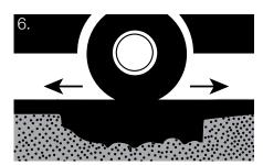
Bitupack surfaces can be used immediately after compaction. A light covering of sand is recommended prior to immediate use.
