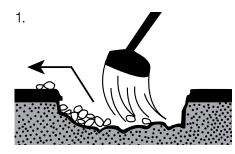
Ensure that the surface area is clean of all dirt, dust, grass, weeds, etc. (if necessary, use a weed killer to inhibit growth).
