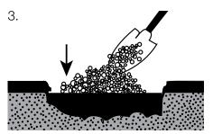
Spread the contents of the bag directly onto the one area. For larger areas, it is recommended that a light coat of emulsion be spread on the base and edges of the area to improve adhesion with the existing surfaces.
