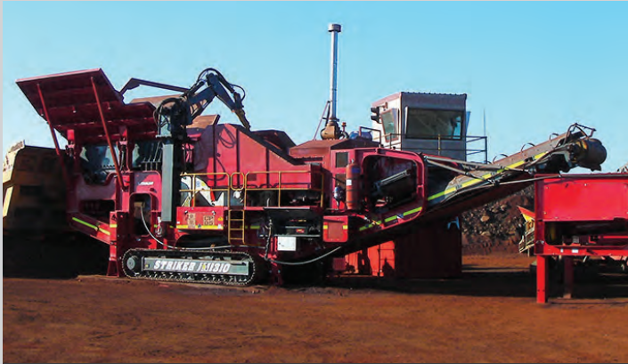
TRACKED JAW CRUSHERS | Up to 900 TPH
