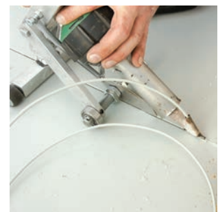
Alkus repair kit - portable welding kit that allows you to join and fix Alkus panels on-site saving valuable downtime.
