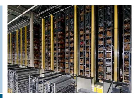
ASRS, or Crane Racking as it is otherwise known, is an efficient and fully automated storage and retrieval system. With narrow aisles and heights of more than 30 metres, this solution offers efficient, high density storage for a large variet of pallets.
