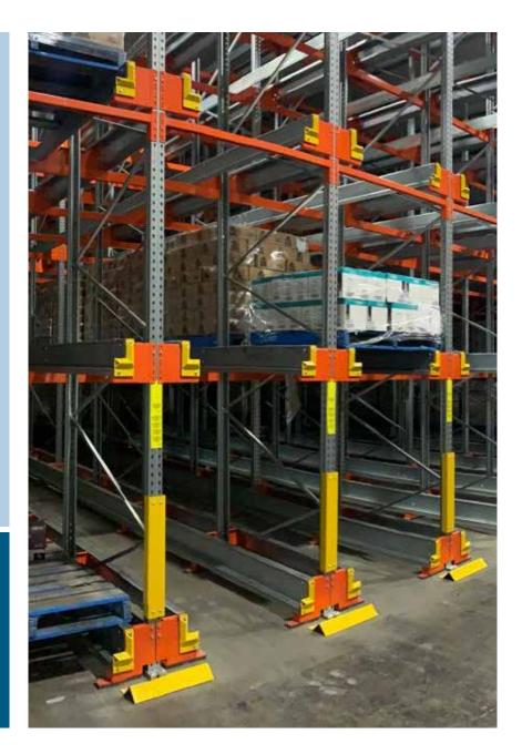
Our Pallet Shuttle system offers a fast, accurate and high density storage solution. The semi-automated system uses a pallet shuttle to deliver and retrieve pallets from within the system, which means forklifts do not need to enter the racking – reducing any risk of damage to the structure itself.
