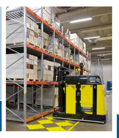
Push-back Rollers – a dynamic storage solution based on the P90 Pallet Racking System and including wheel/roller conveyors. Ideal if you're storing bulk goods on pallets according to the Last-in, First-out (LIFO) principle.
