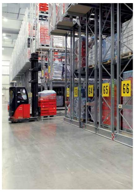
Our Mobile Racking (MOVO) is an electronically controlled, high-load racking system. It runs on in-ground rails with state-of-the-art sensor technology for ease of use and safe operation.
