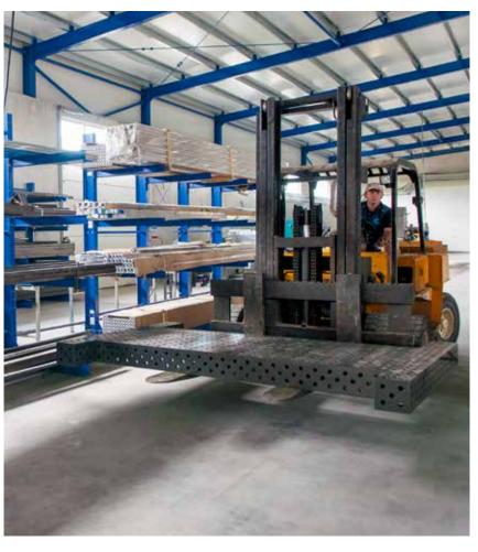
The Medium & Heavy Duty Cantilever is ideal if you need to store long and difficult items such as steel bars, piping, tubes or timber. Storage is horizontal, so can be handled manually or by forklift.
