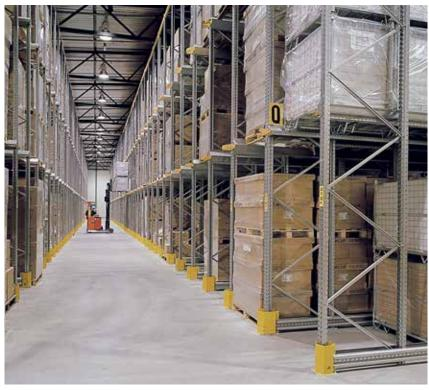
Drive-In pallet racking is very effective for the storage of large quantities of the same or similar products. Our Drive In storage system provide maximum storage capacity with the one of the lowest warehouse footprints.
