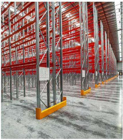
Not only is selective racking the most common configuration for any warehouse, this type of shelving allows for the very best view and accessibility to your stock.
