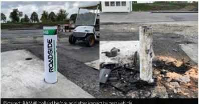
Pictured: RAM48 bollard before and after impact by test vehicle
